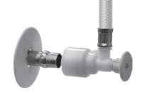
Unique **PUSHON®** design - Nests directly over old brass ferrule simplifying replacement, reducing cost and eliminating in-wall pipe repairs. It can also be used on a pipe without ferrule.
